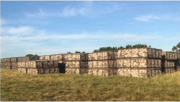
Figure 9 Pre-fabricated reef modules
